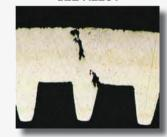
122 Alloy sample 125x magnification. Mounted after 7 days with failure, of accelerated formicary corrosion testing.
